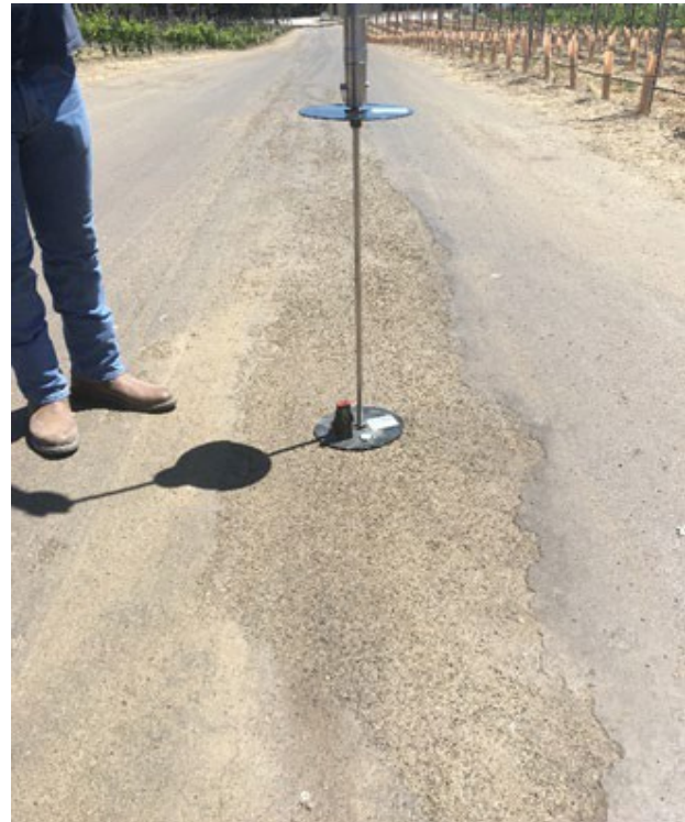
DCP Testing on repaired area
