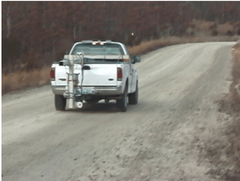
Figure 6. Truck with Mobile Sampler on Treated Road
