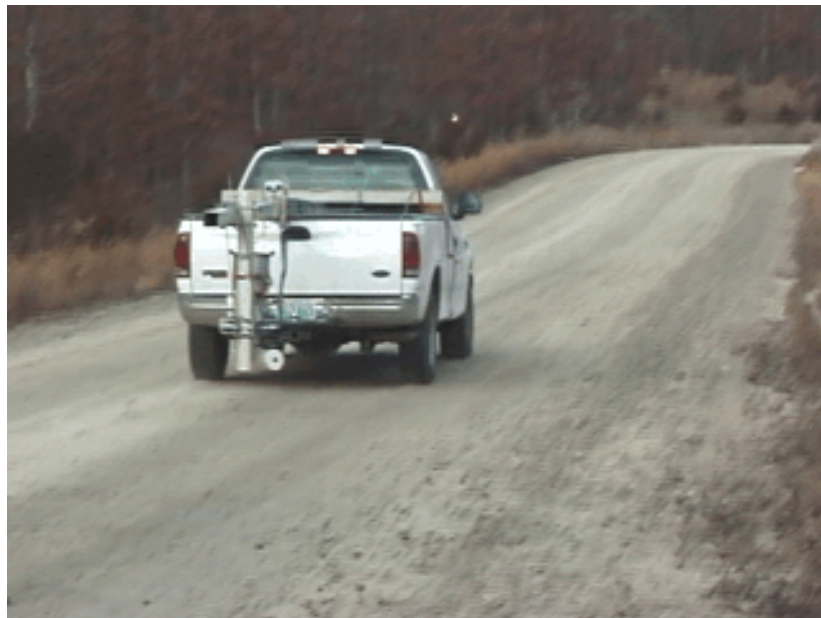
Figure 6. Truck with Mobile Sampler on Treated Road
