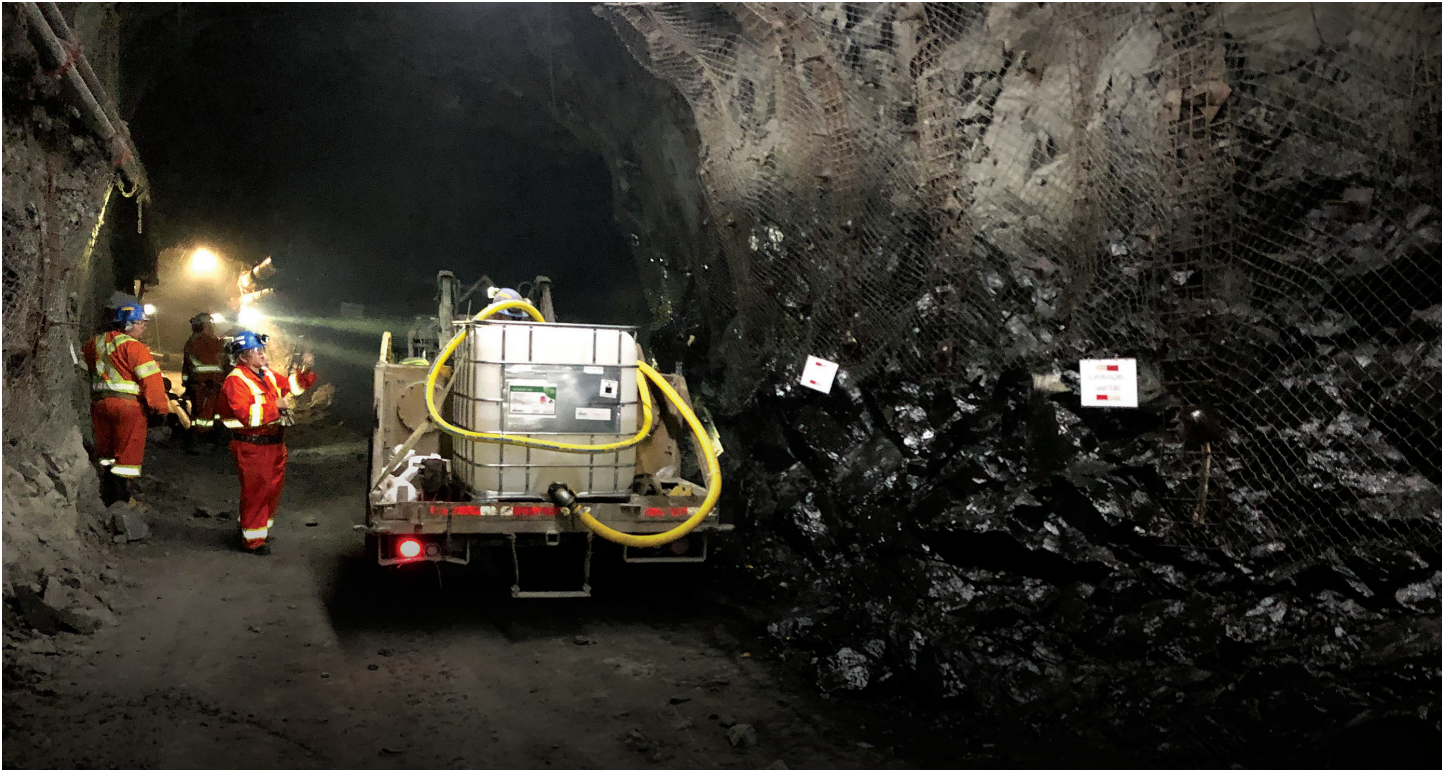
Midwest Industrial Supply's MineKleen Underground Mine Dust Control System. CREDIT: MIDWEST INDUSTRIAL SUPPLY
